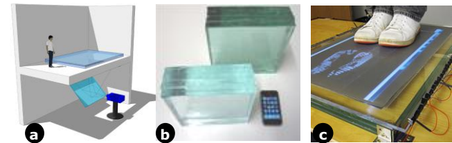
Figure 11: (a) Back-projection design of the floor. (b) Samples of the glass pane. (c) The prototype we use to explore the materials for the final design.
